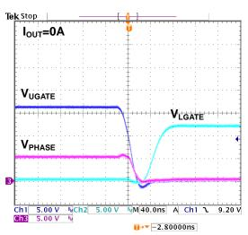
Figure 11. Switching waveform (UGATE falling)
