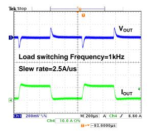
Figure 15. Load Transient Response
