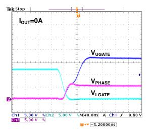
Figure 10. Switching waveform (UGATE rising)
