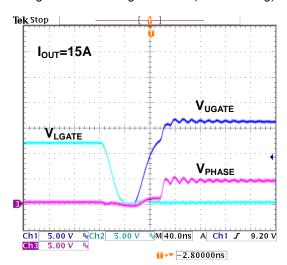
Figure 12. Switching waveform (UGATE rising)
