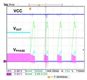
Figure 17. OCP using Dynamic loading
