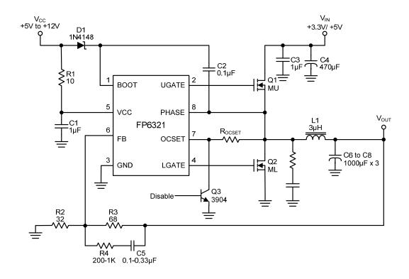
Figure 2. Typical Application Circuit of FP6321
