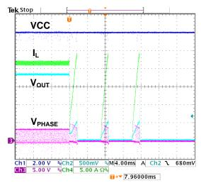
Figure 16. OCP using DC loading
