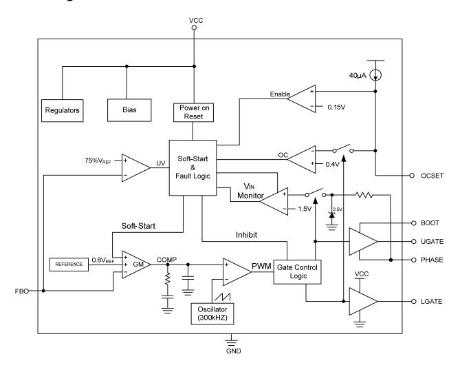
Figure 3. Block Diagram of FP6321
