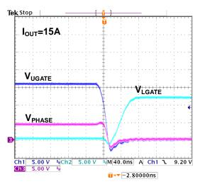
Figure 13. Switching waveform (UGATE falling)
